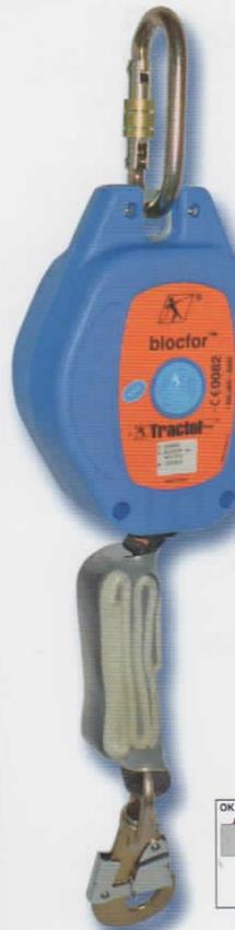
**Blocfor™ 5 and 6 ESD**, automatic fall prevention blocks, are equipped with a new generation of energy dissipator installed at the end of the strap. This new dissipator ensure the user an impact of less than 600 daN even if they fall when the strap is completely unwound. This **ESD** system (**Extremity System Dissipator**) reduces the violence of the impact on the user's body in the event of a fall and protects the strap from the risk of cuts due to sharp angles on terrace roofs.
